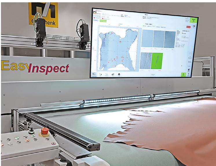
Figure 1. Automated inspection system for finished leather.
