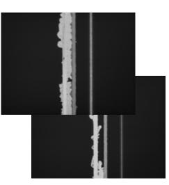
Scribe defects detected with Dr. Schenk SolarMeasure Microscope Station
