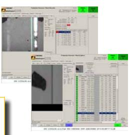
Screen shots: Underscribe (above) and overscribe (below) detected with Dr. Schenk's SolarMeasure Microscope Station
