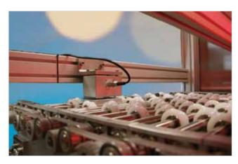
An optional sensor measures the resistivity of the TCO layer on the glass substrate
