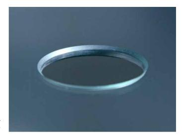
Drill hole in a solar panel backside glass
