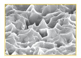
The ideal haze intensity of solar panels' conductive layers will optimize the light trapping effect and thus, the cell efficiency
