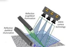
Dr. Schenk MIDA (Mutiple Image Defect Analysis) configuration: single row of cameras, multiple illuminations
